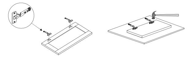
Adjust the hinges and move doors to fill any gaps.
