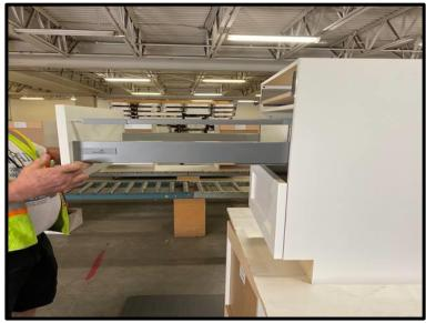
2. With the drawer open, locate the **GREY PLASTIC TABS** on either side and PRESS IN
