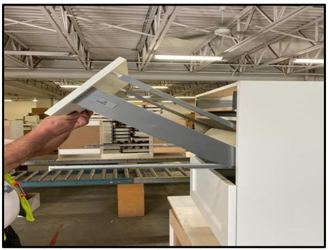
4. To put box back in, leave the slides fully extended and place the box on the slides BACK END FIRST (as shown above) and bring the front of the box down and close the drawer. The tabs will click back into place.
