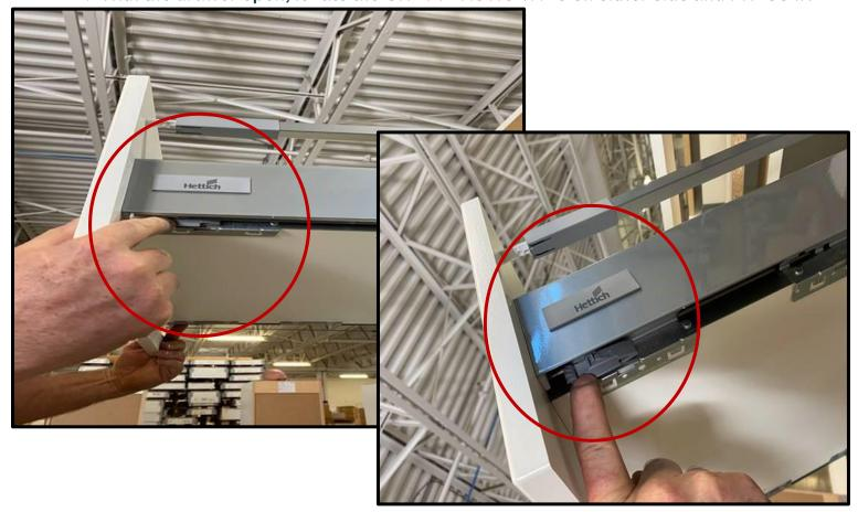
3. While grey tabs are pressed in, LIFT UP the drawer box and remove
